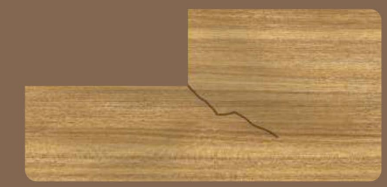
NO CLAIM WILL BE ENTERTAINED FOR CRACKING ARISING OUT OF GROOVE CUTTING OR L SHAPE
